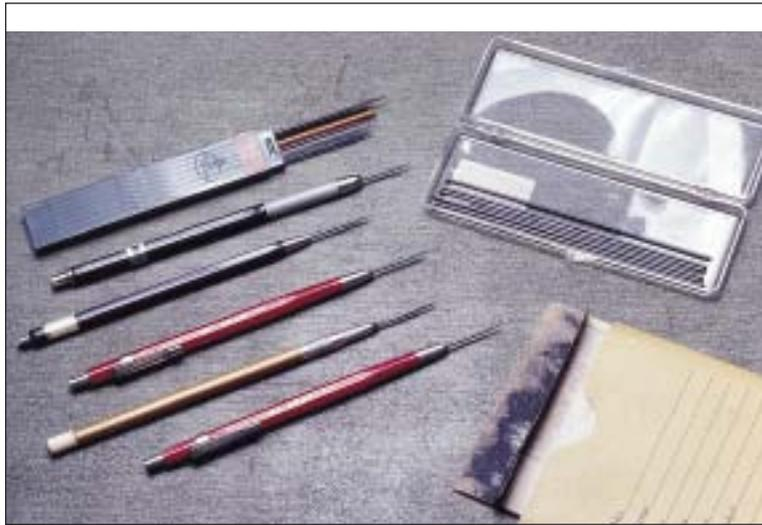
These are some of the various leads used in traditional retouching. They are hard and soft for different applications. Different colored lead holders were used to differentiate lead types. The envelope is fitted with ultra-fine sandpaper for sharpening the leads to an ultra-fine tip.
